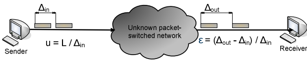
Figure 1. Illustration of end-to-end active probing to obtain available bandwidth estimates. L is the probe packet size and u is the probe-packet rate.
